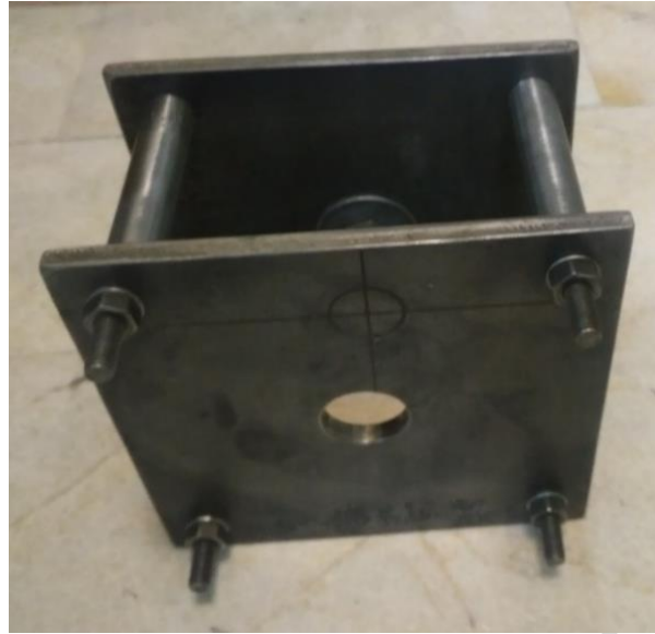
Fig. 5. View of the holding fixture in the impact test facility and how to mark the hit point before installation of the sample
